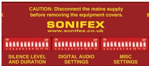
Fig 3-1: RB-DSD8 Rear Panel DIPSwitches
