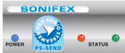
Fig 2-2: PS-SEND Power & Status LEDs
